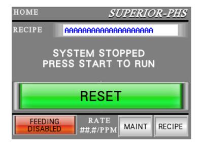
To start the system, first ensure no faults are displayed in red. If a fault is active, perform the corrective action that is noted in the corrective actions section of this document, then tap **"START"** to resume operation.
