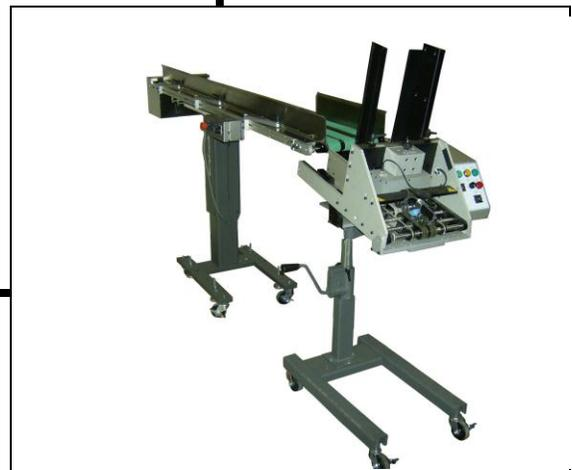
Shown with XM-1 Versatile Friction Feeder
