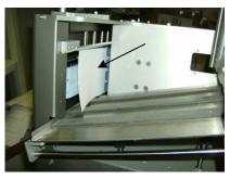
Adjust the tray height so that the product is centered to the feed belt by loosening the adjustable levers, sliding up or down, and tighten the levers.
