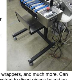
belted conveyors, lugged conveyors, folders, printers, wrappers, and much more. Can be used with virtually any camera, scanner or vision system to divert pieces based on pre-set inspection requirements. Can be used with existing controllers on add-on counting devices, like the **SmartCount™**, to divert a piece on a specified count for manual inspection.
