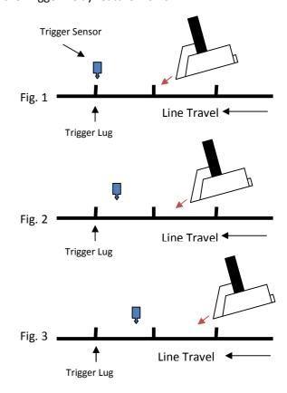
Below you will see a timing chart of how the position of the trigger delay dial will affect each feed cycle. Figure 1 shows full minimum delay, thus an immediate feed cycle once triggered. Figure 2 represents feeding the middle of the pocket – at a line speed of 60 ppm, this dial position would be at ½. Finally, Figure 3 represents offset to the rear of the pocket.
