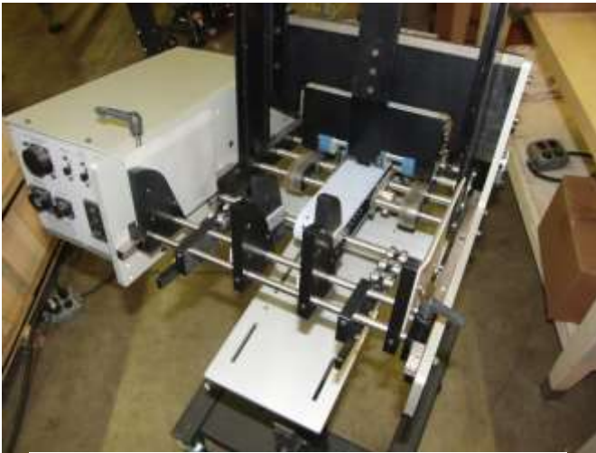
Figure 3.1 Roller Support Wedges and Small Product Wedges in operating position
