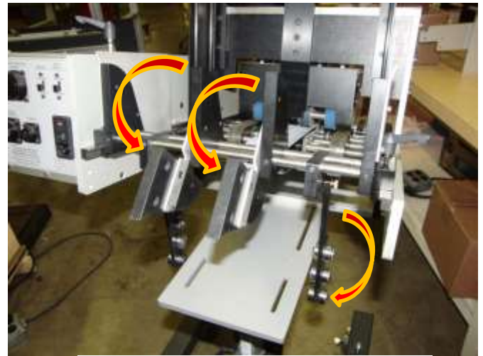
Figure 3.2 Roller Support Wedges and Small Product Wedges disengaged
