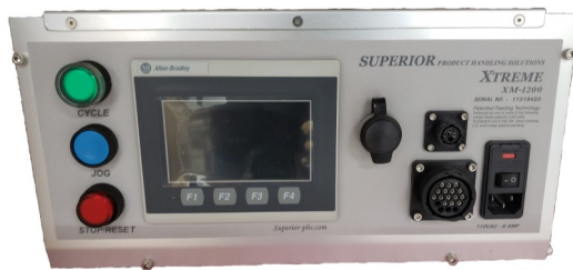
Touch-screen interface, manual controls, and system I/O Interface
